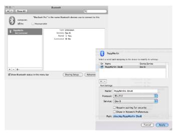
Start Papywizard. Click on "Hardware" -> "Plugins". Select "Merlin-Orion" -> "serial". Click on "Drivers"; paste the previously copied text (CMD + V) in "Serial port". Do not check "Auto-connect". Click on "OK" to validate then click on « Connect » in the main menu. Wait a while.
