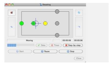
The bottom field indicates whether the motorized head is moving in the stabilization stage or trigger stage along with the time elapsed since the beginning of the sequence.
