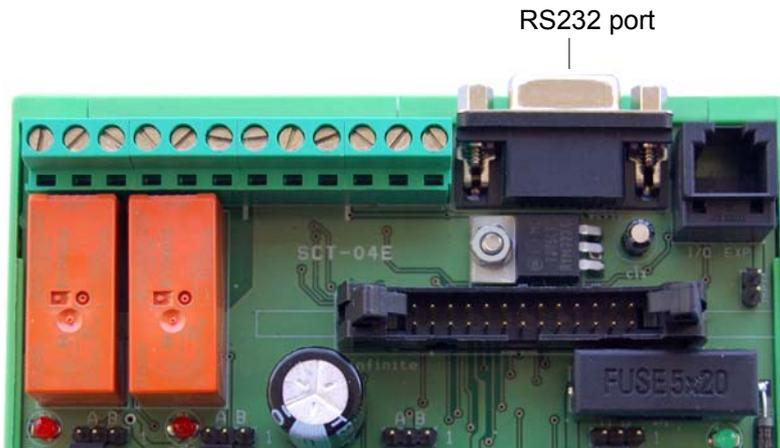
A standard D9 serial cable (straight through) can be used to connect the **auxilliary serial port** with a host computer.
