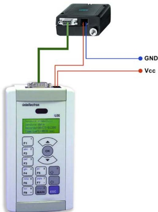
A common modem cable can be used for the external modem connection.
