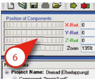
Turn the component into a stable position (also possible in the view by using the mouse).
