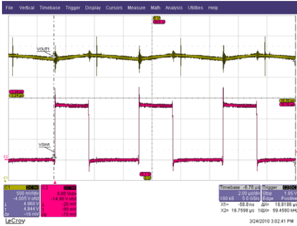
Figure 6. VOUT1 (5 V) and VSW1, 4 A load
