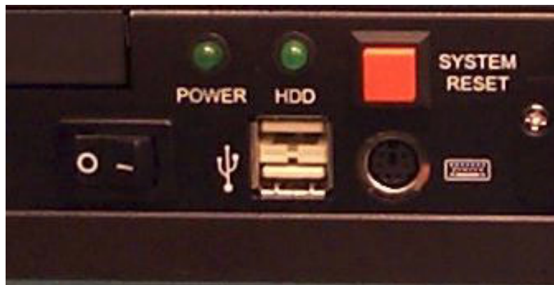
Figure 3.2 Front panel switches, indicators and interfaces
