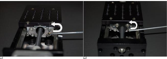
1. Loosen the four screws 1/2 turn on both carriage end 2. Loosen the three screws 1/2 turn on the lead nut plates with a 2.5 mm hex driver. The bearings will with a 2 mm hex driver. The lead nut will have to be automatically re-seat on the rails.
