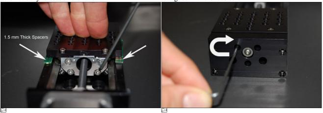
3. Insert 1.5 mm spacers into the gap between the stage 4. Move the stage to its maximum position and tighten top and base. This sets the correct height and the three lead nut screws (0.7 Nm) through the end parallelism of the stage top. Pushing down on the stage plate. This realigns the lead nut with the lead screw top, tighten the four screws on each end plate (2.0 Nm) where it is constrained at the thrust bearing.
