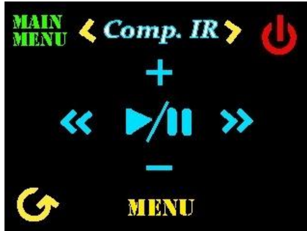
Figure 14: Computer Infrared controller screen. Each button can be programmed to learn an infrared code.
