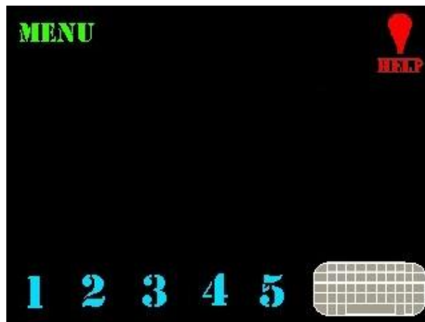
Figure 13: Mouse interface state. Changes of touch on this screen are sent to Bluetooth as a mouse change command. This has a menu button for personalizing this state, help button, shortcut buttons and the keyboard changes the state to the keyboard interface state.
