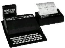
It comes with a joystick interface and the tape speed can either be 300 bps or 4200 bps. It has 4 KB ROM and 2 KB RAM (expandable to 16KB).
