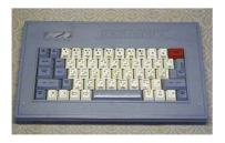
Over 15,000 Hobbits (or Hobetas) have been produced in St.Petersburg since 1993. The Hobbit was mostly used in schools. It comes with two 5.25 inch disk drives, networking, three joystick ports (two Sinclair and one Kempston), 74-key full size keyboard with programmable function keys, built in assembler/disassembler, Centronics printer port, RS232 serial port, video output to both composite video (TV) and TTL (EGA) and 64K RAM. It runs a version of CP/M called "Beta".
