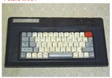
A russian ZX Spectrum clone from around 1993. Size is 14 x 7.2 x 2 inches. The name suggest that it has 64 KB of RAM and was made by Peters Plus Ltd that now makes the Sprinter.
