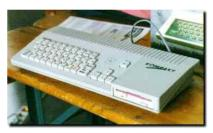
The Didaktik Kompakt is a Didaktik M with a built-in 3.5" disk drive that uses non-standard MS-DOS formatted disks at 840 KB. It has standard connectors for joysticks and printer and a built-in parallel interface using i8255 as in Didaktik Gama. All other features are the same as Didaktik M.
