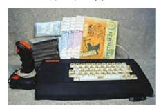
The size of the system unit is 14 x 8 x 2 1/2 inches, the weight is 1.5 kg approx.
