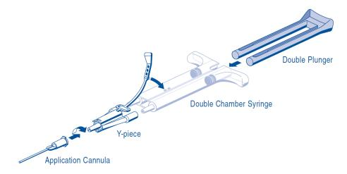
Device Set Instructions: firmly connect the double chamber syringe nozzles to the Y-piece and secure it by fastening the tether strap to the syringe. Fit an application cannula onto the Y-piece. To avoid clogging, do not expel the air remaining inside the Y-piece or application cannula until application.
