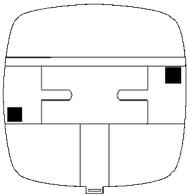
To remove meter, pull down on Release Clip.
