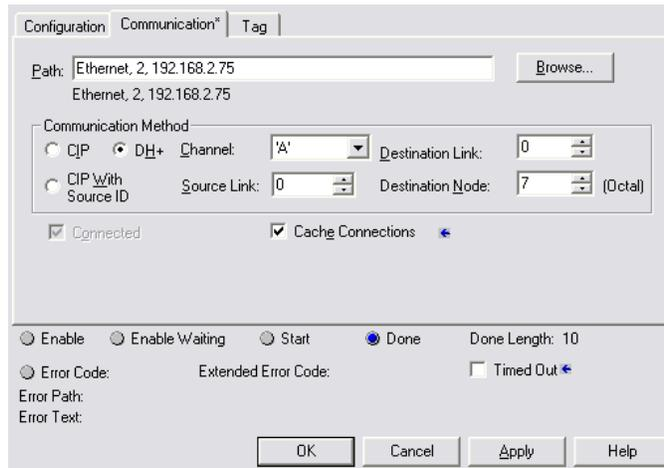
If using a SCADA or DCS software application to poll for data, setup the message as though it is communicating through a ControlLogix Bridge.
