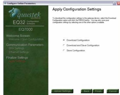
If you encounter any issue downloading the configuration, just press the Reset button on the left hand side of the unit, ( or power OFF/ON) let it cycle through, then press the configure button on right hand side, then click on Finish to download the configuration file.
