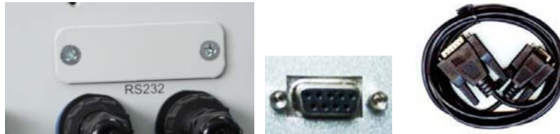
Fig. 17 RS232 serial port and special RS232 cable
