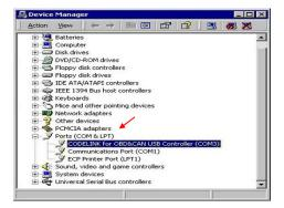
Click 'Port (COM & LPT)' you will see 'CODELINK for OBD&CAN USB Controller (COM3)' the CreaderV has been connected at COM3.
