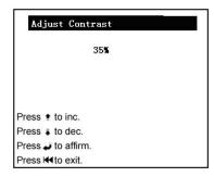
In the [Adjust Contrast] interface, you can adjust the contrast of screen. Press [ ] to increase contrast or press [ ] to decrease contrast according to you desired.
