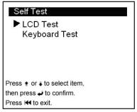
Select [LCD Test] and press [  $\clubsuit \overline{\phantom{a}}$  ] to enter the LCD test interface as shown below:
