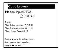
You can use [ ] [ ] | key to change the first letter. It can be switched among "P", "B", "C" and "U". And press [ ] moves the cursor to next. And then press [ ] [ ] | key to input number. After you input the code number, press [ ] to view the definition of the code.
