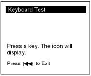
You can press [ 1], [ ] or [ ]. If they appear on the screen, it indicates that the Button is normal and you can use them for testing. If there isn't any icon appearing on the screen, please contact Launch for repair.
