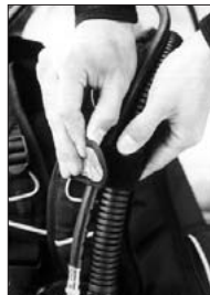
(Fig. 2) Secure the airway together with QD Hose to the Hock & Loop hose retainer.
