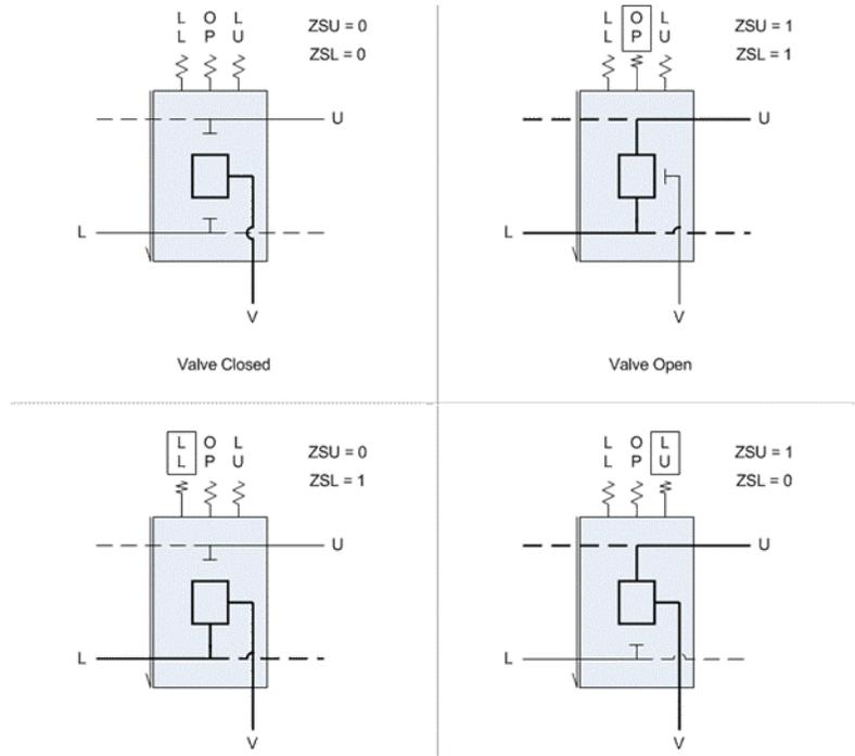
In the closed position (all outputs off), flow is not directed anywhere and the valve cavity is vented to waste recovery. In the open state, flow is directed from the upper line to the lower line. In the Lower Lift position, flow is directed from the lower line through the valve cavity to waste recovery. In the Upper Lift position, flow is directed from the upper line through the valve cavity to waste recovery.
