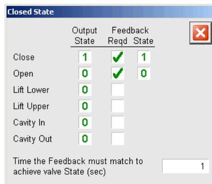
**TIP** You can open the state configuration message boxes for multiple states at the same time. This can make it easier for you to check your selections against the documentation for your particular valve and actuator.
