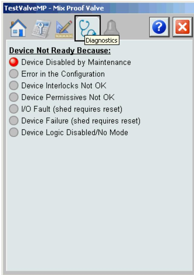
The figure above shows that the valve is not ready because the device has been disabled by Maintenance.
