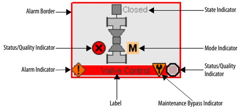
Each display element includes a touch field that accesses the object's faceplate. In addition, there is a tooltip that displays the object's configured tag and description.
