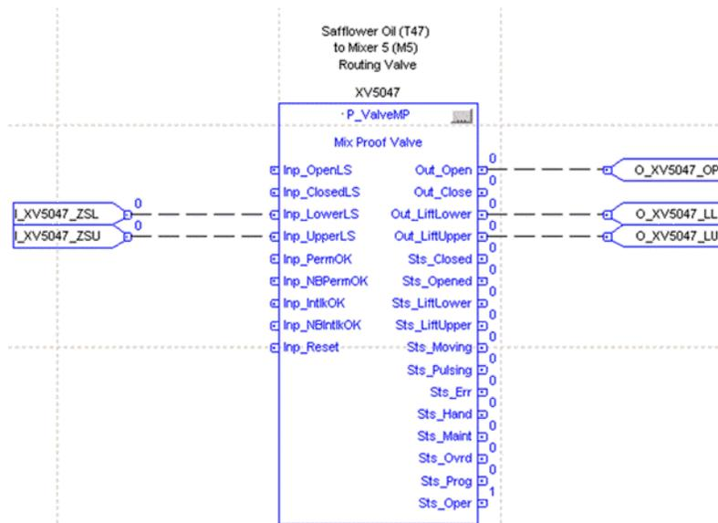
The two limit switches from the field are connected into inputs Inp\_LowerLS and Inp\_UpperLS. The three outputs to the field are connected to Out\_Open, Out\_LiftLower, and Out\_LiftUpper.
