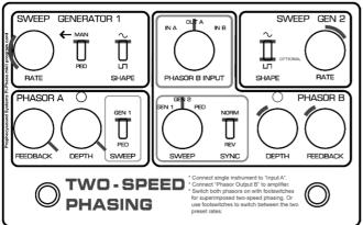
Using this setting you can switch PHASOR A and PHASOR B on or off to create a phased signal with two different modulation types layered, or with the audio processed by a single phase section.
