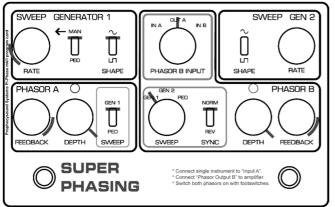
The signal from [PHASOR B OUTPUT] is processed by all 12-phase stages within your Pi-Phase mk2 for the deepest and most lush sound; note that both PHASOR A and PHASOR B are modulated by the same control signal, that being GEN 1. Experiment with different settings within this program, for example turning the [FEEDBACK] controls of both PHASOR A and PHASOR B down to minimum, or by adjusting the [DEPTH] controls for both sections for a more subtle effect.
