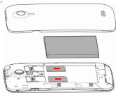
3. Finally insert the battery and replace the rear cover of the mobile phone.
