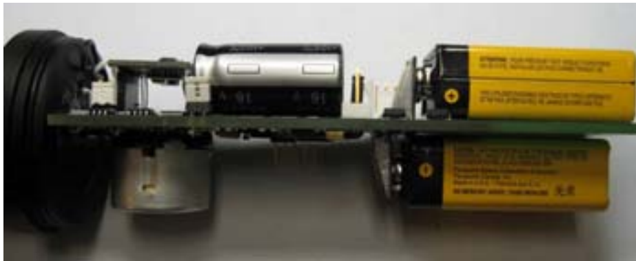
Figure 4-3 ATT-400 Battery Installation
