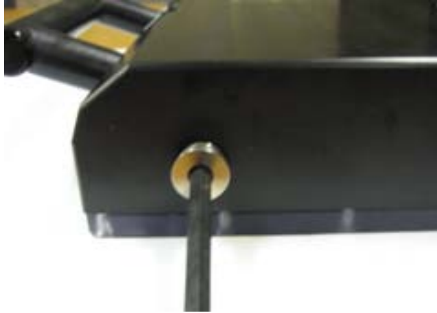
Figure 3-3 Charging Port Plug Removal
