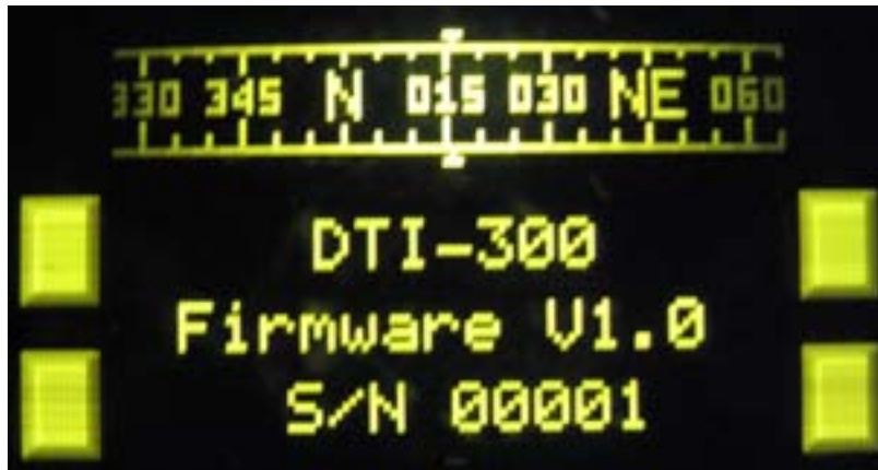
Figure 4-7 DTI-300 HEADING display mode
