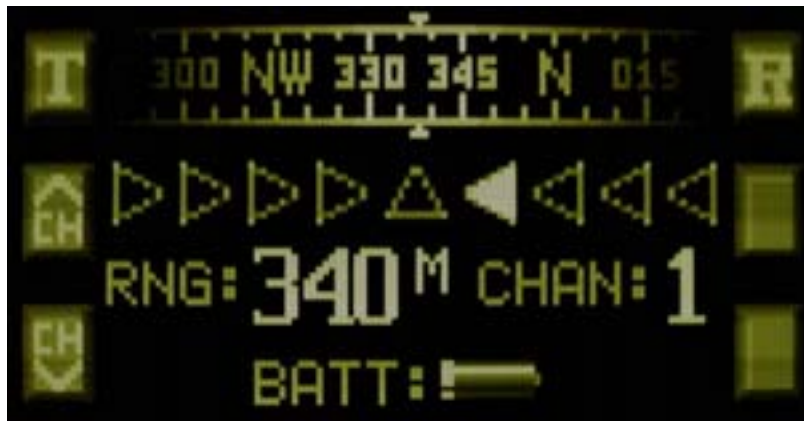
Figure 4-6 DTI-300 NORMAL Operation display mode
