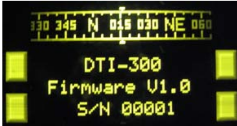
Figure 3-7 HEADING display mode
