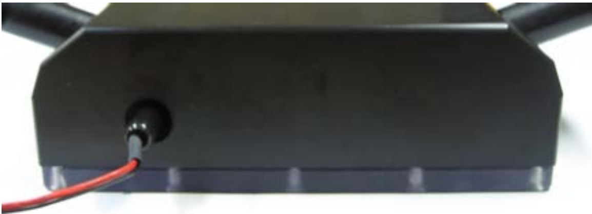
Figure 3-4 Charging Connector to DTI-300
