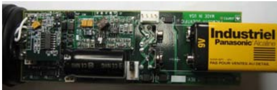
Figure 4-2 ATT-400 Battery Connections
