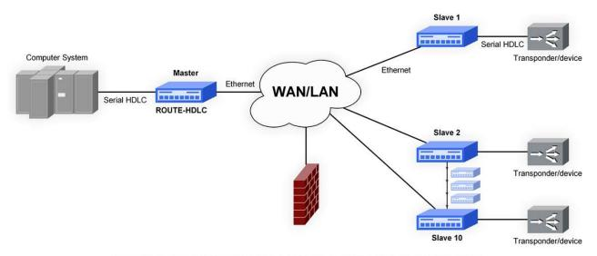
The system can support up to 10 Slaves and 500 Transponder/devices.
