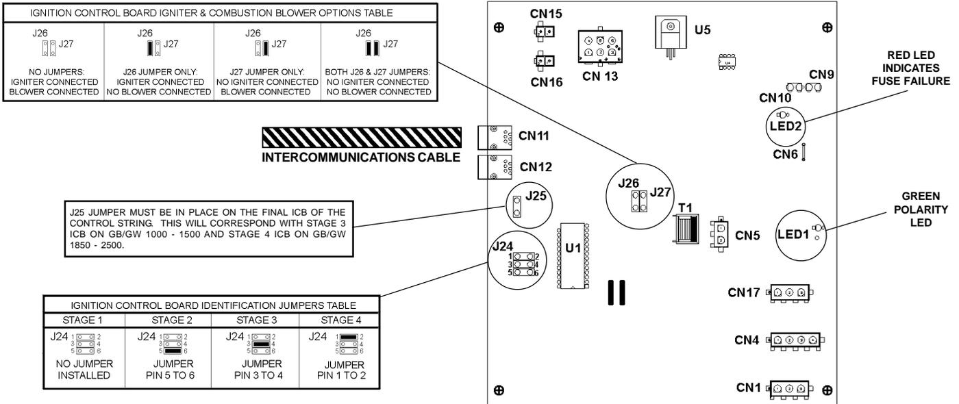
Figure 2. Jumper Configurations for Ignition Control Board.
