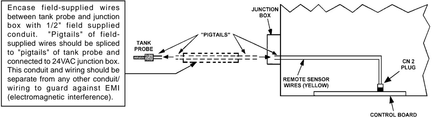
**Figure 5. Tank Probe Installation**
