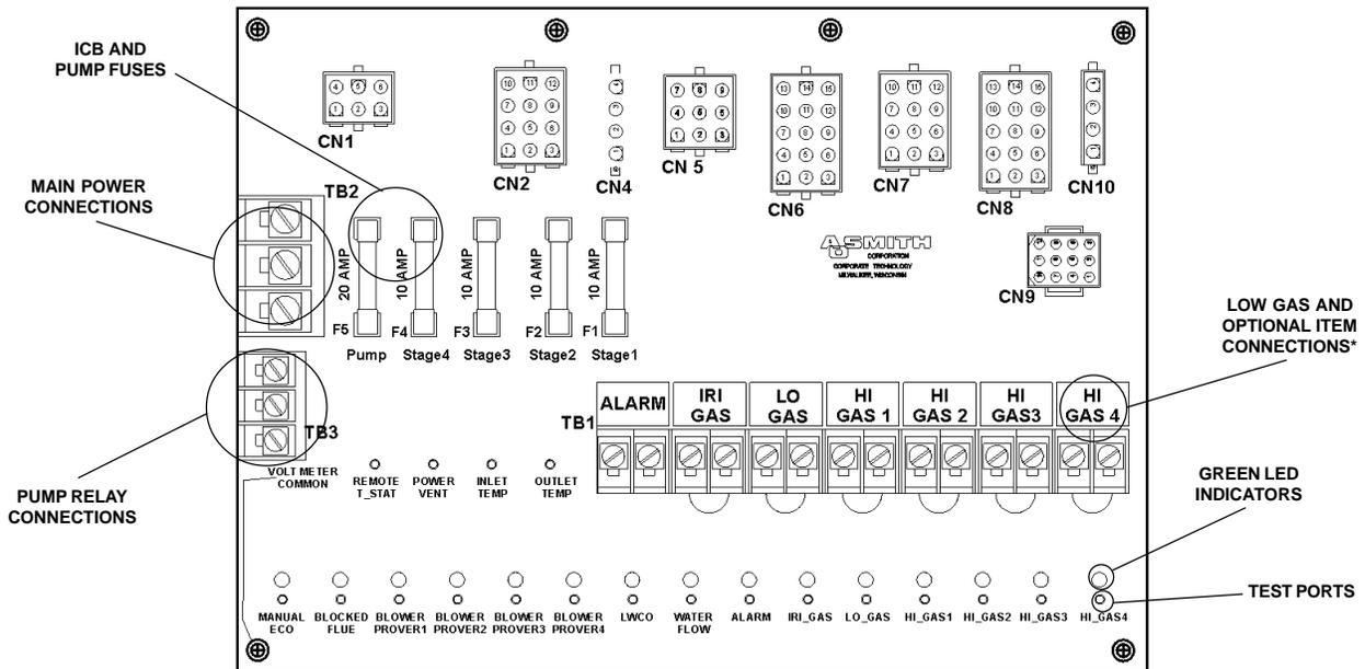
Figure 3. Interface Board Components.
