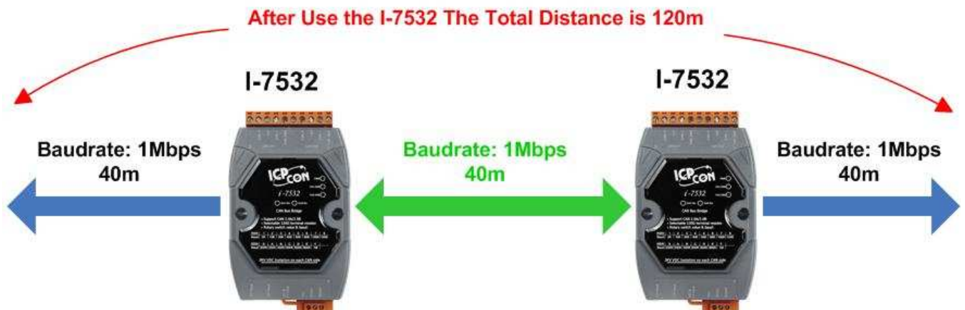
Figure 1-2 Application of I-7532 Extend Distance.
