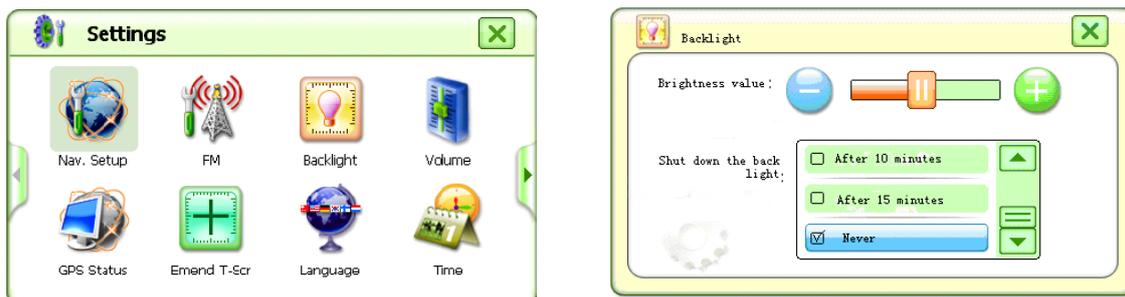
Through this option, the brightness and duration of backlight can be configured. When completing setup, click the icon
