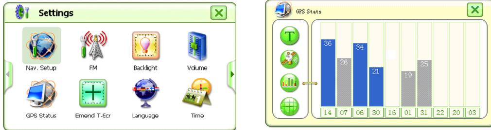
Grey means the GPS is receiving the satellites and not position yet, as shown as below:
