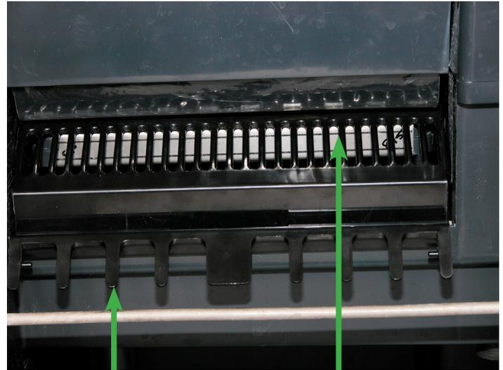
Front view of freezing compartment, right arrow points to Spray Platform, under the Cube Deflector. Push curtain back and check that it is in this position.
