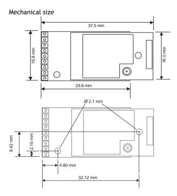
There are two holes available for mounting. The one nearest the connection pads can accept an M2 screw or American equivalent #0-80. Important Note: DO NOT USE #2 screw size. Note that the mounting hole is connected directly to the Battery ground of the acquisition module.
