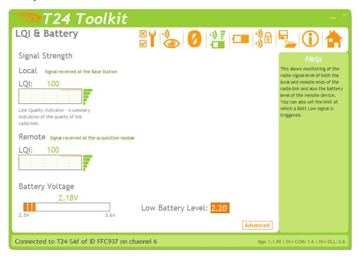
Here you can see the voltage of the battery and the radio signal levels at the base station and the remote acquisition module. This simple view gives an LQI value which stands for Link Quality Indicator. This value will range from 0 to 100 and within this band you should still achieve communications. As the level drops towards zero communications may become intermittent but still achievable.
