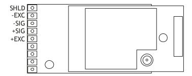
The resistance of the strain gauge can be between 85 and 5000 Ohms. The T24-SAf can support up to 4 3500hm strain gauges bridges attached in parallel (At the expense of reduced battery life).
