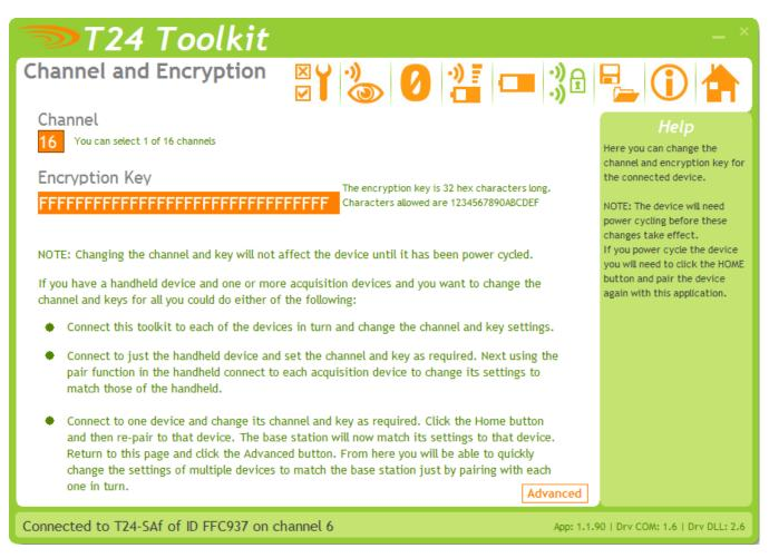
Here you can change the channel and encryption key for the acquisition module device. Simply pair to the T24-SAf and change its channel and key.
