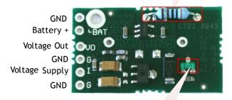
LED lights when supply voltage applied
