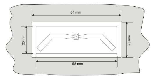
The bulkhead mounting antenna can be used with metal or plastic housings. Care must be taken when mounting the Antenna to ensure the installation does not become directional.
