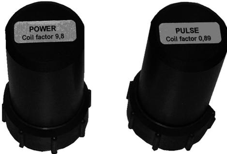
INA 702 becomes a single turn loop when fitted with the **PULSE** plug, which allows the generation of pulsed field strengths up to 1200 A/m, where the current is generated by a 4400 V surge generator.
