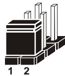
Jumper Block 1-2 pin close(enabled) Looks like this
