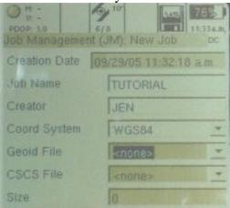
II. Then press the Menu button and select "Save". Give the Leica GS20 a minute to process your request.
