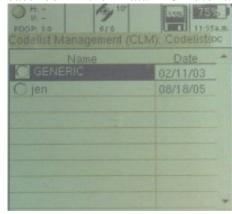
IV. An error message saying that the job does not contain any data shows up; select "Ok". The GS20 will automatically open the new feature window to start collecting data.
