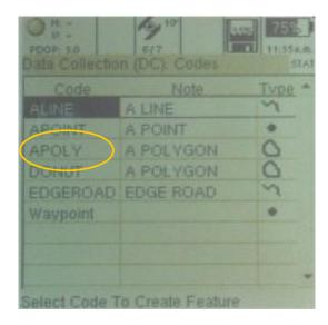
2. Collecting data for a polygon is similar to collecting line data. The data can be collected as either a stream or as nodes. To start collecting data select "occupy" and collect the points. When finished select "Stop" and/or "Done."
