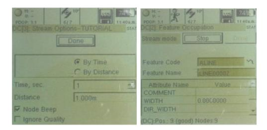
c. Using the "Node" selection: Click "Occupy" and then click Enter where you would like a node on the line to be. When the GS20 has collected the node that you want, select "Save Node", similar to collecting points. When the line is complete, select "Done."
