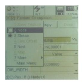
b. Using the "Stream" selection: When you select stream, a menu will appear that allows you to select how the GS20 collects the data. Set the GS20 to collect either by time or by distance, and the interval. Then click "Done." Click "Occupy" and walk the path for which you would like to collect data. When done, click "Done."
