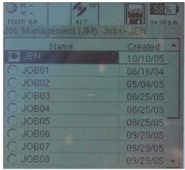
3. To create a new job press the Menu button and select Create New Job. Then just fill in the information as described in the Collecting Data section that follows.
