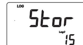
By pressing the STORE key a complete set of information is memorized: date, time, EC or TDS and temperature readings.
