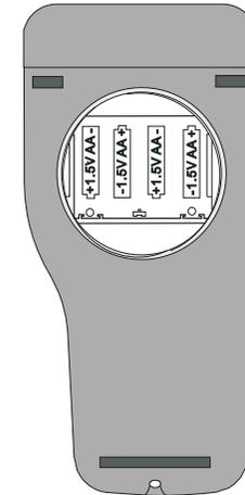
**Note:** When batteries are removed, the meter can remember date & time for about 5 minutes. After that, it will be necessary to set again date & time through the setup procedure.
