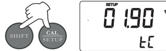
Select the desired setup item using the arrow keys, then press CFM to select and edit the setup item. The current value of the selected item starts blinking (if the parameter can be modified).
