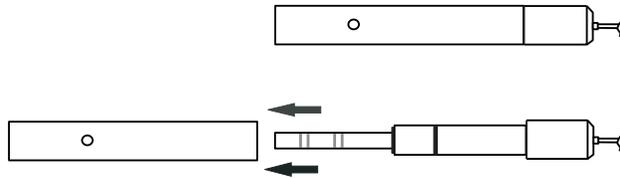
After cleaning the probe, recalibrate the instrument.
