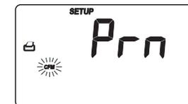
Press CFM to print the setup report or CAL to exit without printing.
