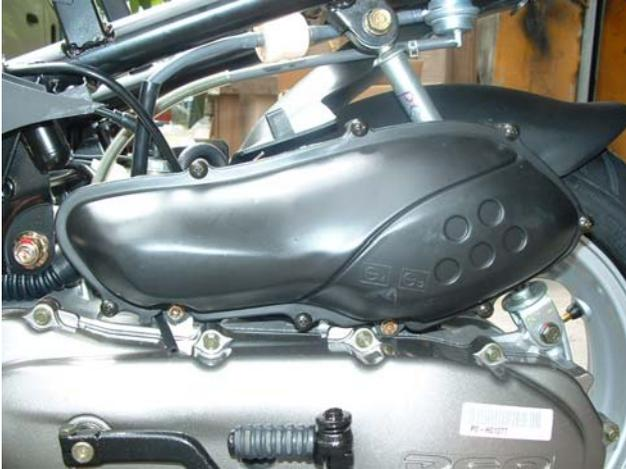
PREVENT THE ASH ENTERING THE ENGINE AND WEAR OUT THE ENGINE. PLEASE ASK THE DEALERS TO CHECK & CLEAN THE FILTER FOR THE TIME BEING.
