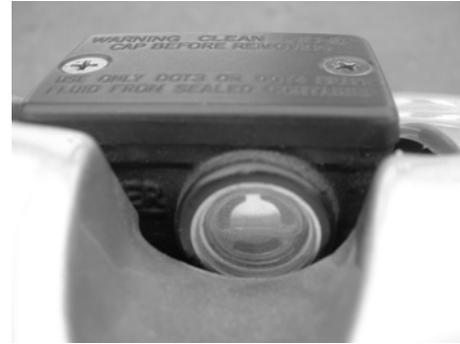
1. WHEN CHECKING THE OIL LEVEL, PLEASE TURN THE HANDLE BAR ASSURING THAT THE BRAKE OIL IS IN HORIZONTAL POSITION.
