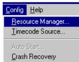
**Timecode Source...** Opens the timecode display selection dialog box. If the record channel has more than one timecode track, this allows you to select the one for display in the record and playback panels.
