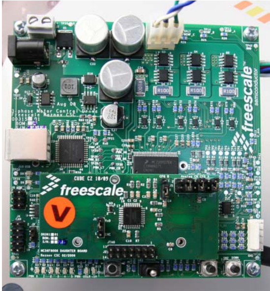
Figure 4-2. 3-Phase BLDC/PMSM Low-Voltage Motor Control Drive Board with Daughter Board
