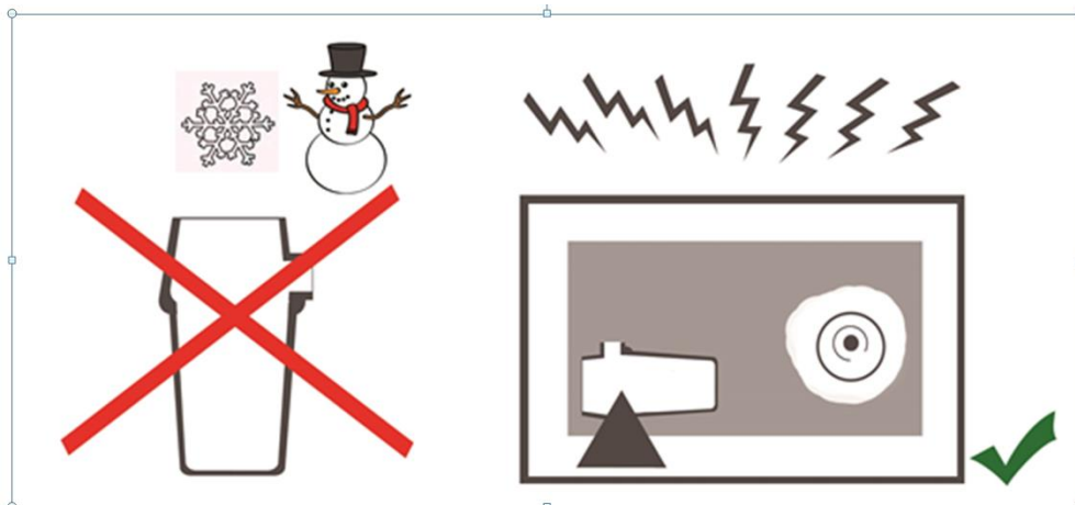
Fig. 5: Pre-heating the crucible in cold ambient temperatures
