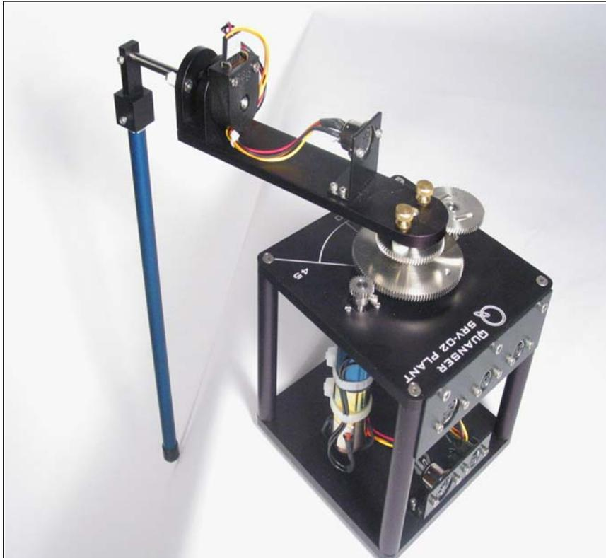
Figure 1 - SRV02 with a ROTPEN Module
