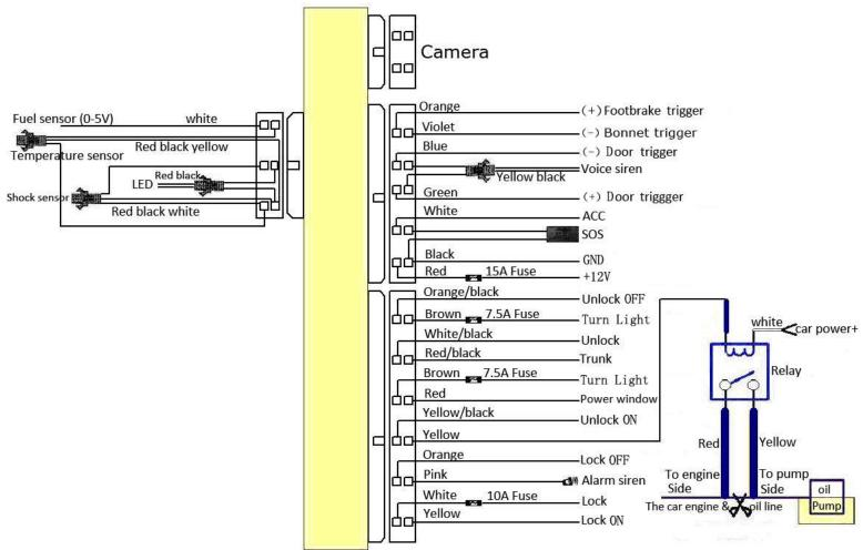
**6.2.2** Central locking system wiring diagram
