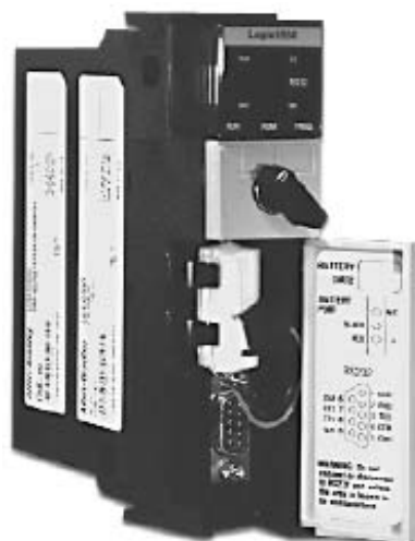
Figure 33 - Allen-Bradley ControlLogix Controller
