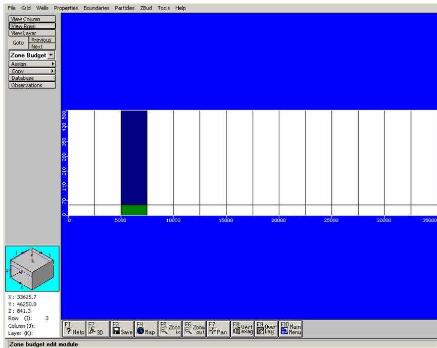
In cross section view, you can see that Zone 2 was assigned to the cell in the upper layer, and Zone 3 was assigned to the cell in the lower layer
