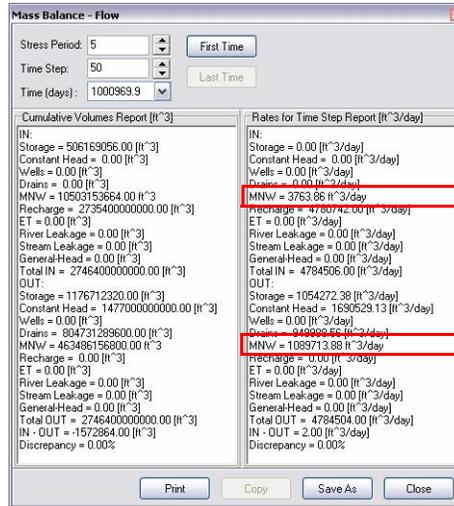
Multi-node wells appear in the mass balance as the “MNW” term. Mutli-node wells occur in both the inflow and the outflow portions of the mass balance. The total rate of outflow from multi-node wells was 1,089,713.88 ft<sup>3</sup>/day and a total inflow was about 3,786.86 ft<sup>3</sup>/day, which yields a net discharge rate of 1,085,950.02 ft<sup>3</sup>/day.
