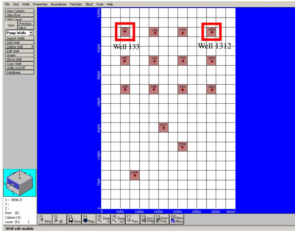
The two multi-node wells are indicated in the image above. Both MNW wells are screened across both the top and bottom aquifer. This can be seen by viewing a cross section of this row. To do so,
