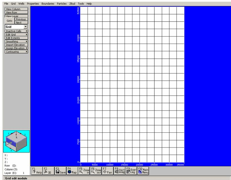
This image displays the grid of the model; as you can see, the model domain is 21 rows by 14 columns, by 2 layers. Cell size is 2,500 x 2,500 feet. Total area is 66 mi<sup>2</sup>.
