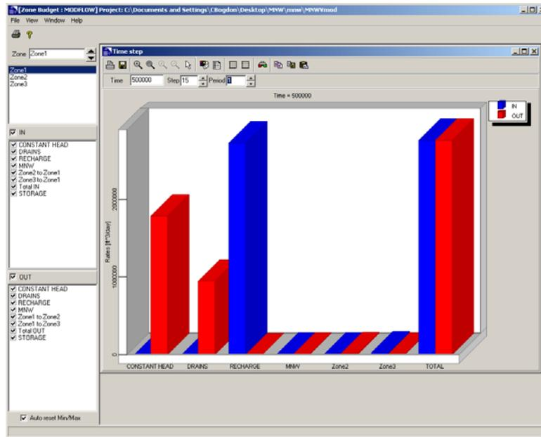
This graph plots a bar chart of the flow IN and OUT of the system of the selected zone through the individual sources and sinks (flow boundary conditions and storage) for selected output times.
