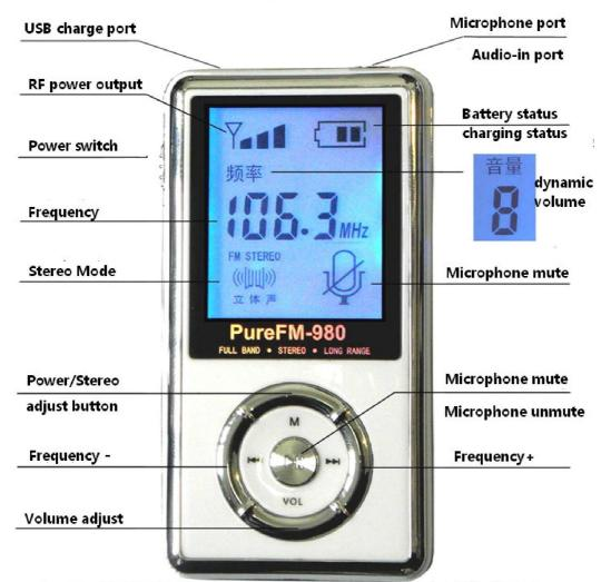
1. RF power/Stereo mode adjust: Press M button, in the following 2 seconds:
