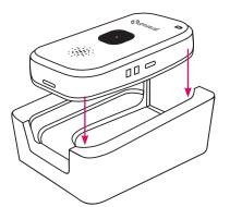
Inserting the Splash into the Charging Cradle
