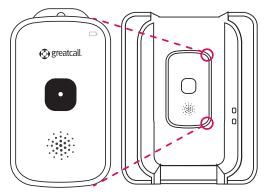
Aligning the Splash with the Charging Cradle
