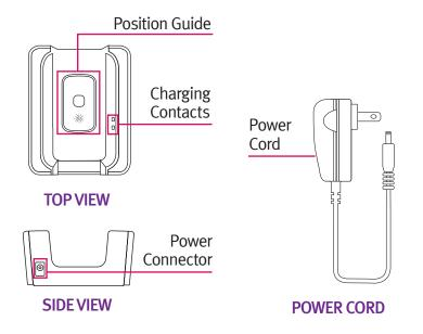
**Position Guide** – Shows you how to position the Splash in the Charging Cradle.
