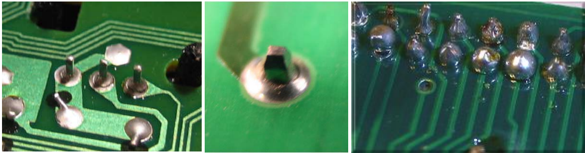
Figure 33: photographs of bad soldering (courtesy of T-Minus)
