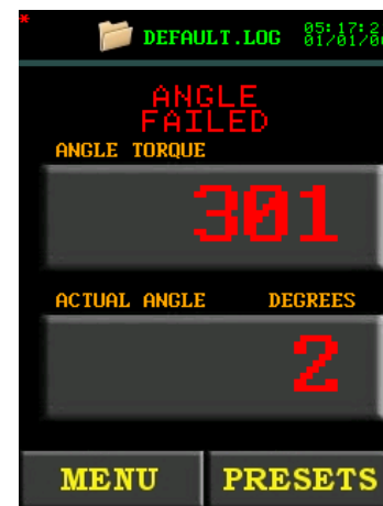
Figure 5.4.1-2: Failed Torque and Angle Cycle
