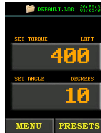
Figure 4.3.7-2: Main Screen with New Set Torque
