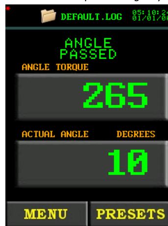
Figure 5.4.1-1: Passed Torque and Angle Cycle
