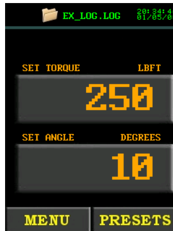
Figure 4.3.2-8: Main Screen with New Data Log Displayed
