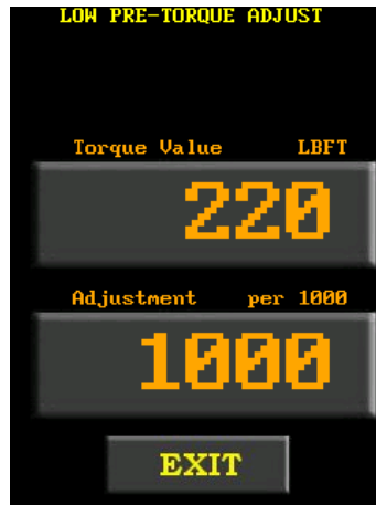
Figure 4.3.23-8: Low Pre-Torque Adjustment Screen
