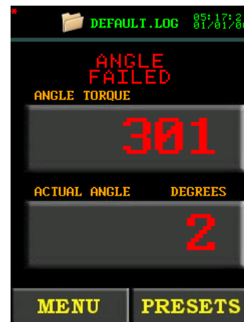
Figure 5.4.2-3: Failed Torque and Angle Cycle
