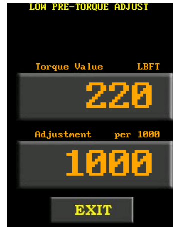
Figure 4.3.23-4: Low Pre-Torque Adjustment Screen
