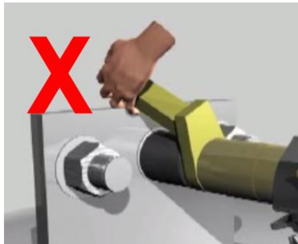
Figure 5.1.1-2: Incorrect Placement of Hand/Body Parts During Operation
