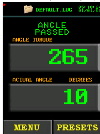
Figure 5.4.2-2: Passed Torque and Angle Cycle
