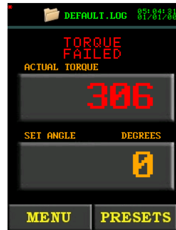
Figure 5.2-2: Failed Torque Cycle
