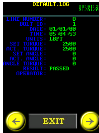
Figure 4.3.3-2: View Cycle Logs – Passed Cycle
