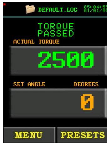
Figure 5.2-1: Passed Torque Cycle
