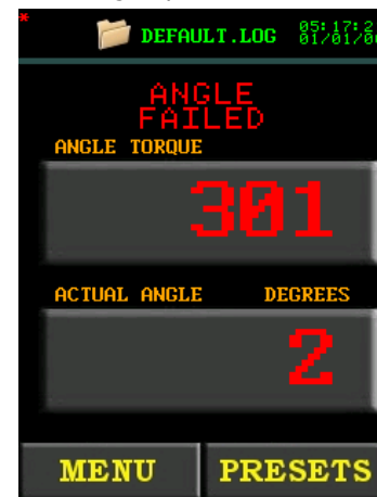
Figure 5.3-3: Failed Angle Cycle
