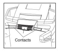
To measure your heart rate, stand on the foot rails and hold the pulse bar with your palms on the metal contacts; avoid moving your hands. When your pulse is detected, a heart symbol in the calorie display will flash each time your heart beats, one or two dashes will appear, and then your heart rate will be shown. For the most accurate heart rate reading, continue to hold the contacts for about 15 seconds.
