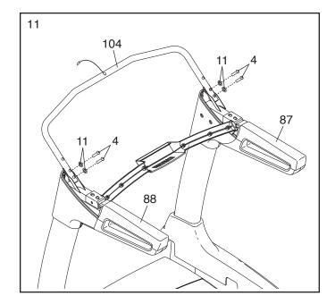
12. With the help of a second person, hold the console assembly near the Left Handrail (88).
