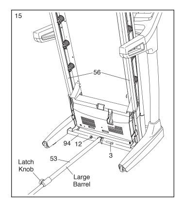
16. Attach the upper end of the Storage Latch (53) to the Frame (56) with a 3/8" x 1 3/4" Bolt (6) and a 3/8" Nut (12). Note: It may be necessary to move the Frame (56) back and forth to align the Storage Latch with the Frame.
