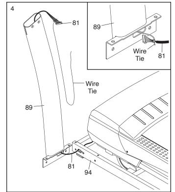
5. Hold the Left Upright (89) against the Base (94). **Be careful not to pinch any wires.** Insert two 3/8" x 2 3/4" Screws (7) and two 3/8" x 1 1/4" Screws (8) with two 3/8" Star Washers (13) into the Left Upright.
