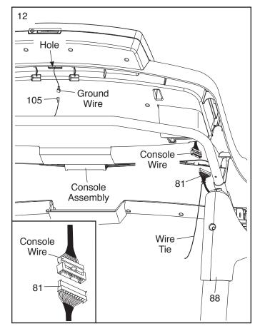
13. Set the console assembly on the Left Handrail (88) and the Right Handrail (87). Be careful not to pinch any wires. Insert the excess Upright Wire (not shown) into the Left Handrail.
