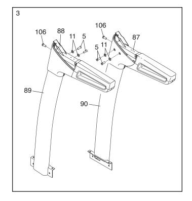
4. Identify the Left Upright (89), which is marked "Left." Have a second person hold the Left Upright near the Base (94).
