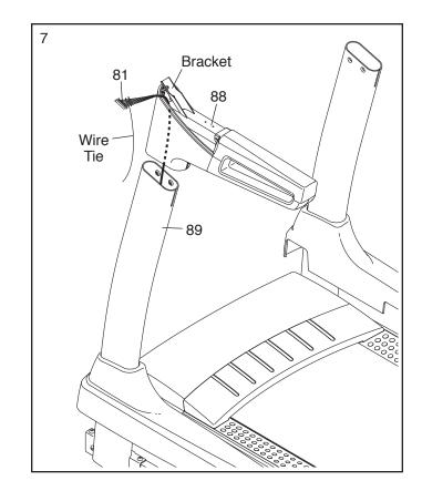
8. Attach the Left Handrail (88) to the Left Upright (89) with the two 5/16" x 1" Screws (5), two 5/16" Star Washers (11), and the 5/16" x 1 1/4" Bolt (106) that you removed in step 3. **Do not fully tighten the Screws and Bolt yet.**
