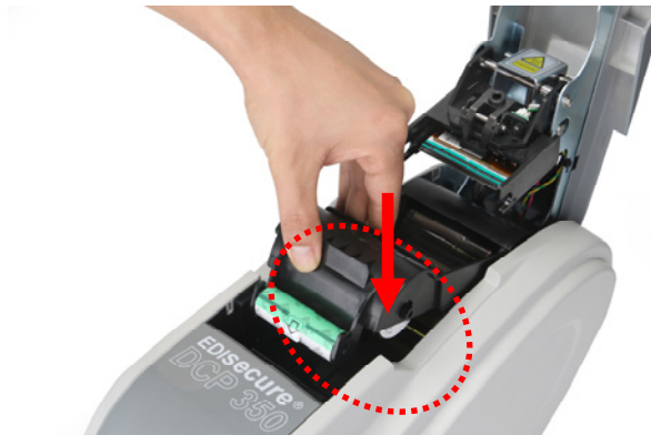
Pic.12 Installing the ribbon cartridge
