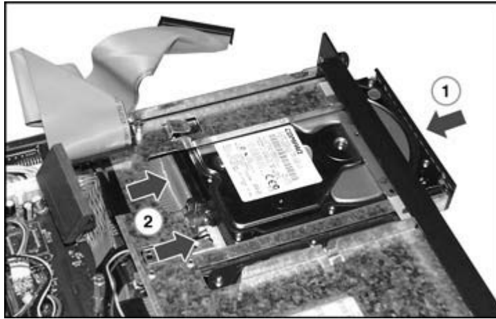
Figure 4-32: Connecting power and media cables to the second SCSI drive
