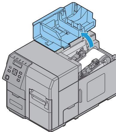
3. Pull the front cover open lever at the paper feed slot.
