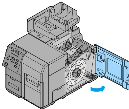
4. Pull out the roll paper flange while holding the release lever of the roll paper flange between your fingers.
