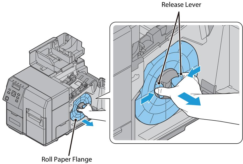
5. Attach the roll paper to the spindle, and push the core of the roll paper as far as possible so that it is securely fit it into place.
