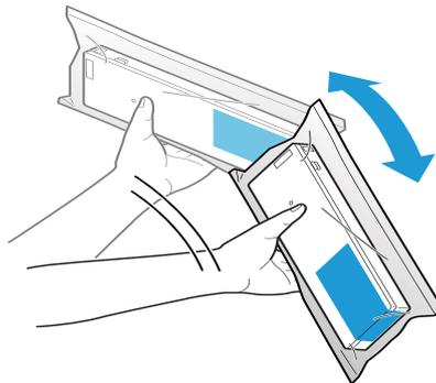
4. Push all the ink cartridges of the four colors gently into the product until they click in place. Check the color of the ink cartridge label and of the ink cartridge holder label, and set the cartridges to each matching color.
