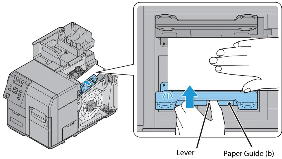
11. Adjust the guide panel of the paper guide (b) so that it aligns perfectly with the edge of the paper.
