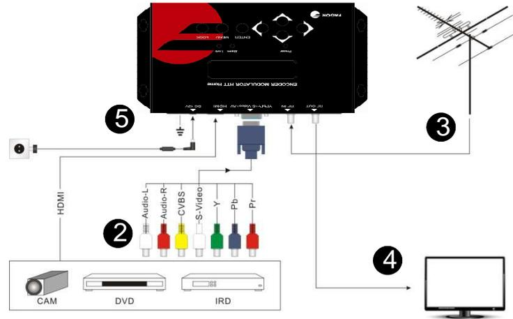
5. Power supply connection: a) Connect the earth cable; b) Connect the power plug to the unit mains connector; c) Connect the power plug to the mains socket.
