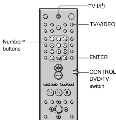
Press and hold TV I/O while entering your TV's manufacturer's code (see the table) using the number buttons and press ENTER. Then release TV I/O.
