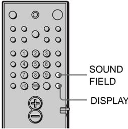
Press **SOUND FIELD** repeatedly until the sound field you want appears on the front panel display.
