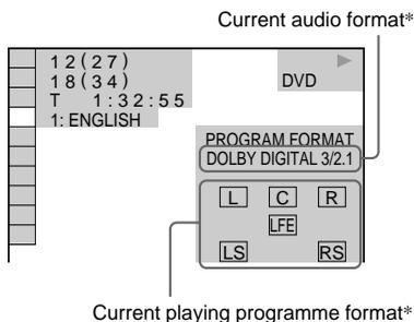
\*“PCM,” “MPEG,” “DTS,” or “DOLBY DIGITAL” is displayed. For “DOLBY DIGITAL,” the channels in the playing track are displayed numerically as follows:
