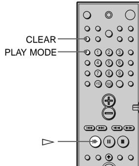
**1** In stop mode, press PLAY MODE repeatedly until “SHUFFLE” appears on the front panel display.
