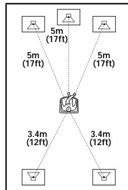
Be sure to change the value in the Setup Display when you move the speakers. The default adjustments are in parentheses.
