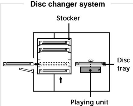
The disc changer consists of a playing unit, trays which hold the discs, and a stoker which transports the discs on their trays to the disc slot and the playing unit.
