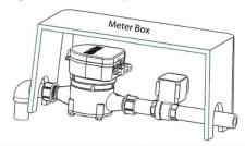
NOTE: The HydraMeter is water tight as long as either a cable, or the supplied grommet plugs are inserted into the three black grommets at the front of the HydraMeter, and those grommets are tightened appropriately. While our valves are also watertight, neither the valves nor the HydraMeter are intended for continuous submerged use. Hence, if water is anticipated to continually enter and flood the meter box, the installation of the HydraMeter and valve should be above ground.
