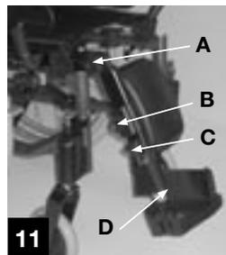
The footplate is height adjustable : loosen the knob (C), adjust to the desired height based upon the preset holes and tighten firmly.
