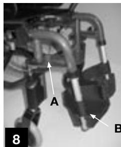
Push lever (A) sideways and swivel towards outside or inside in case there is not enough space. (To return to the initial position, align the footrest support, it locks automatically). To remove the footrest support, simply pull it up after unlocking the assembly.
