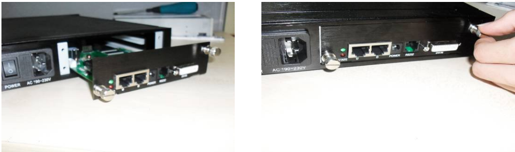
Fig. 4.1 Sending card installation
