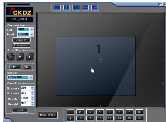
Fig 5.15 Accurate coordinate of capture window
