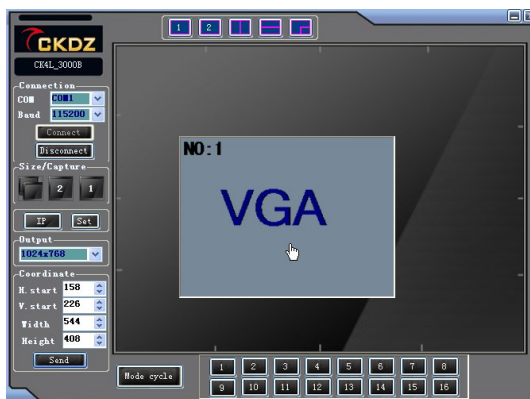
Fig 5.14 Accurate coordinate of normal window
