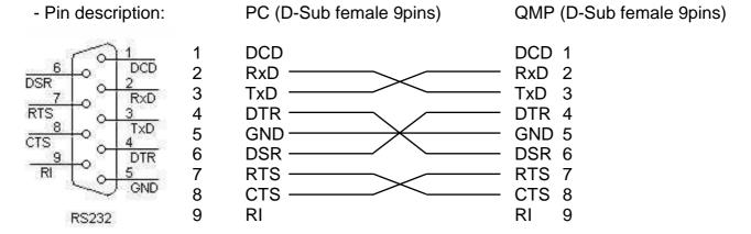
A cable between the PC and the QUORION QMP cash register has two 9-pin female D-Sub connectors.
